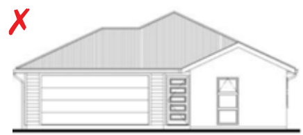
Unacceptable gable & hipped roof
