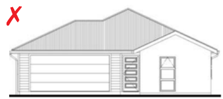
Unacceptable gable & hipped roof
