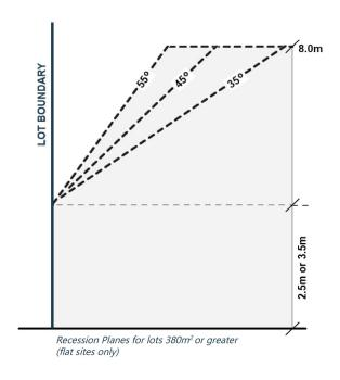
A flat site is defined as 'a site where the ground slope is equal to or less than 6 degrees (i.e. equal to or less than 1 in 9.5). Ground slope in relation to building height shall be determined by measurement over the extremities of each building elevation. Where all elevations indicate a ground slope of less than 6 degrees (i.e. equal to or less than 1 in 9.5), rules applicable to flat sites will apply.'
