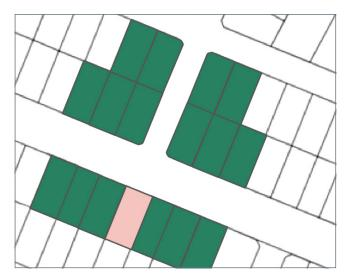
Section layout demonstrating identical façade rule.
