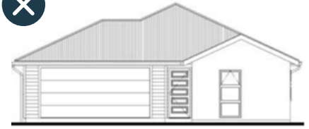
Unacceptable gable & hipped roof
