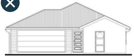
Unacceptable gable & hipped roof
