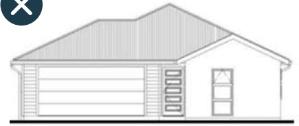
Unacceptable gable & hipped roof
